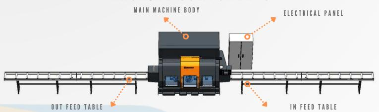
The main machine has become 4 groups brushes, each group has included in top and bottom brushes. The machine has 8 brushes in total, each brush is provided with single and vertical movement for quality surface of extrusion profiles. All brushes speed adjustable by inverter on the PLC screen for synchronization.
